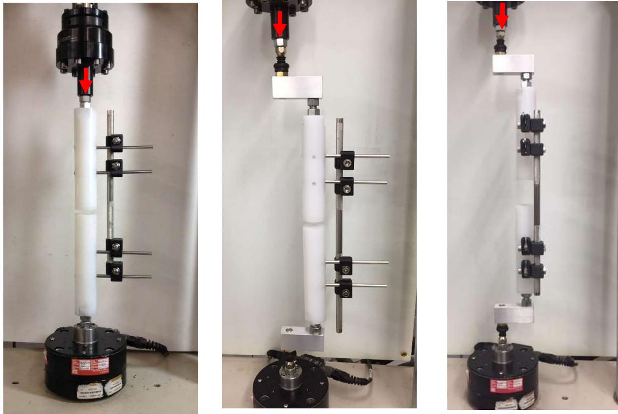
**Fig. 4** Left to right: **a** Axial compression, **b** Over ball-and socket, AP-bending test set up providing an offset of 50 mm to the axial force **c** Over ball-and-socket, ML-bending test set up with a perpendicular force transmission. The direction of input force is denoted by the red arrow shown
