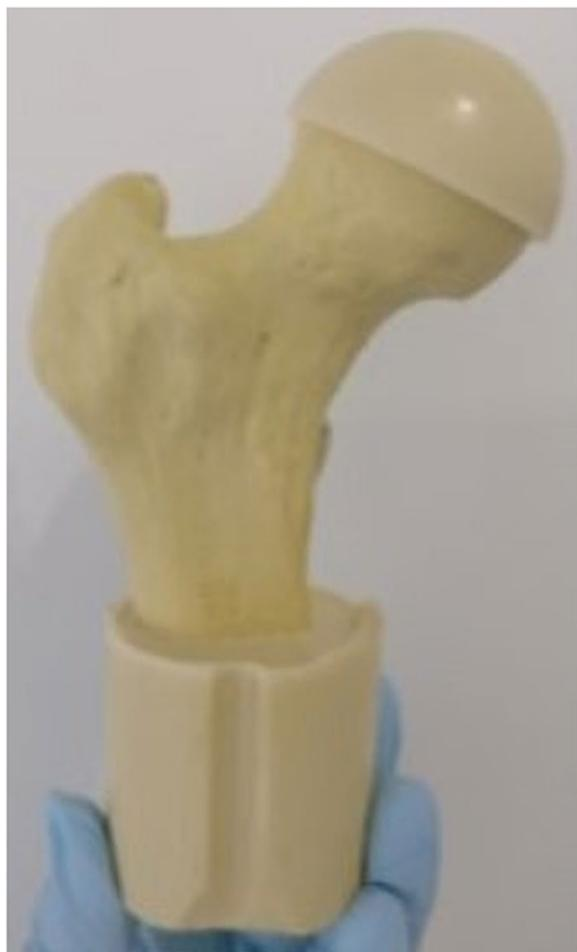
**Fig. 2** Embedded truncated generic Femur in preparation for  $\mu$ -CT scanning
