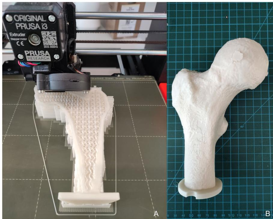
**Fig. 5** Printing Process and finally 3D printed bone example (Femur1). **A** Example of a 3D printed bone during the printing process with support. The variable cortex thickness with 100% linear infill is shown as well as the gyroid pattern which represents the artificial spongiosa. At the distal end, a plate was added to place the bone before embedding. **B** final 3D printed bone after removal of the supporting structure
