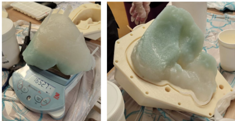
Fig. 9 Silicone rubber liver model showing the green color as the tumor
