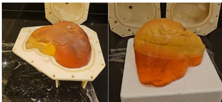
Fig. 10 The ballistic gel model in its mold (left) and the full liver model with a visible red tumor (right)
