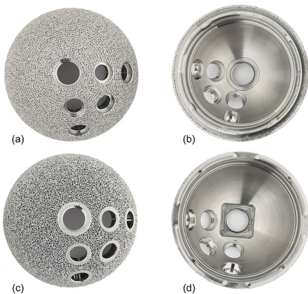
Fig. 1 Macroscopic images showing an example of the two designs analysed: (a and b) the back and front sides of the Trident I shell and (c and d) the back and front sides of the Trident II shell
