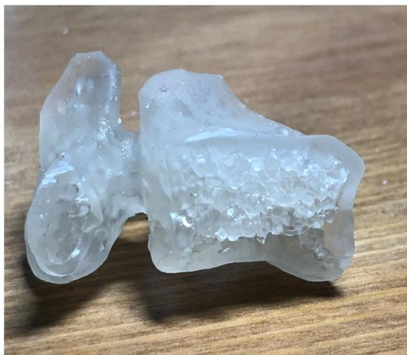
**Fig. 1** Section cut of 3DP vertebrae showing internal mesh trabecular structure while housed within a thick cortical wall, attempting to model real bone. Code was written to add a stochastic framework of a mesh within a thick wall while the model was printed with 100% Clear® resin off the Form 2® SLA Printer
