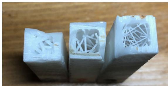
**Fig. 7** 3 of 10 cubic blocks tested for structural mechanical characteristics. Differences in cylindrical diameters, cortical wall thickness, and gap sizes between cylinders can be seen between the 3 prints
