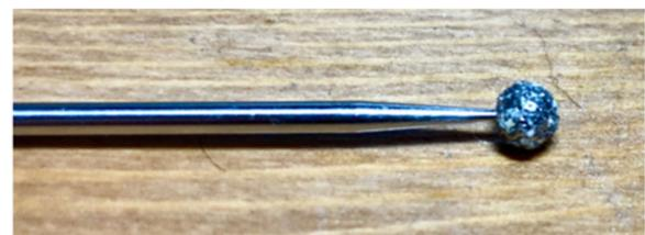
**Fig. 5** 5-mm diameter diamond-coated bur tip used in all tests. This bur tip is common in orthopedic and neurosurgery
