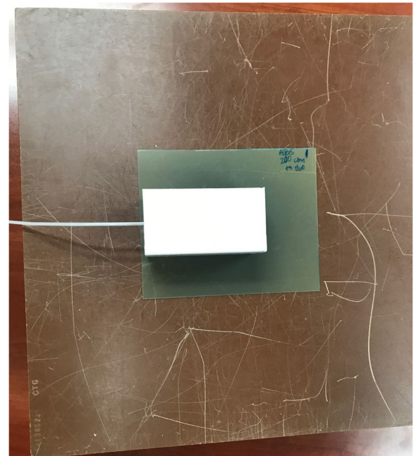
Fig. 3 Film is placed 3 cm from the catheter and source, below the 3D printed block
