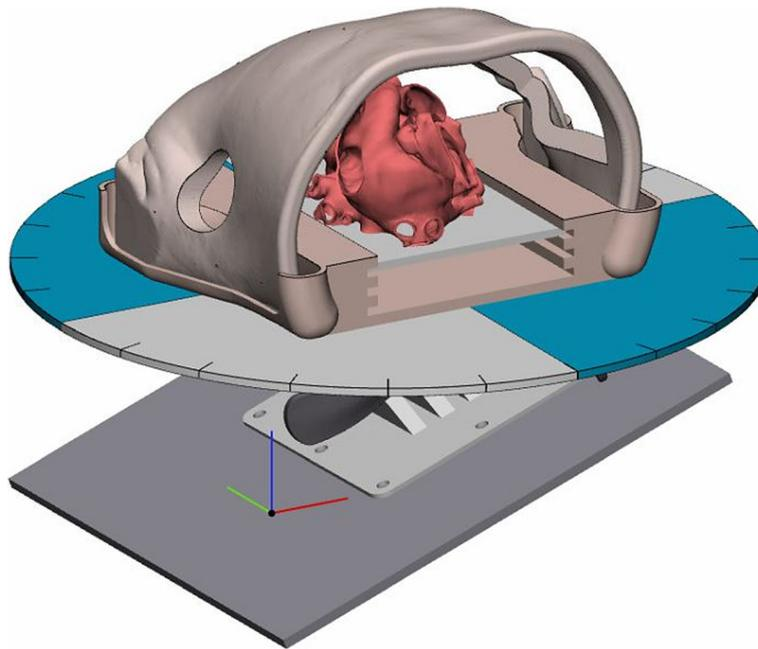
**Fig. 5** Computer render of a minimally invasive dynamic chest wall and operating table simulator. Note the absence of a median sternotomy incision and the inclusion of a mini-thoracotomy incision the surgeon will operate through. The opposite side of the chest is removed to allow the teacher to observe the performance of the surgeon
