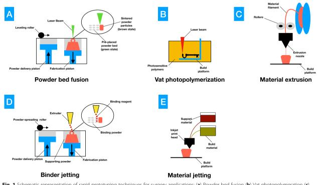
Fig. 1 Schematic representation of rapid prototyping techniques for surgery applications: (a) Powder bed fusion (b) Vat photopolymeration (c) Material extrusion (d) Binder jetting (e) Material jetting
