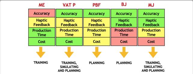
Fig. 5 Advantages (green) and limitations (red) of different 3D printing technology to create 3D anatomical models. These characteristics lead the choice for the best 3D printer technique for every clinical or academical purpose
