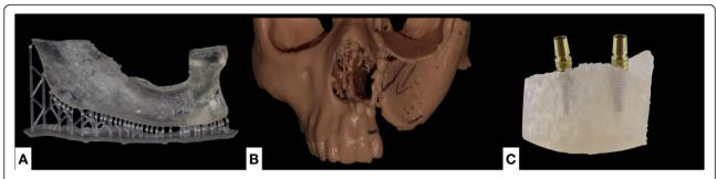
**Fig. 2** Examples of anatomical models fabricated by Additive manufacturing. A: A mandible model fabricated using SLA to serve as a template for bone allograft preparation during surgery. B: A model fabricated using SLA to visualize the extent of a bone defect (cleft) for planning the bone reconstructive surgery. C: A model representing a section of a mandible. It was used for training students in dental implant surgery
