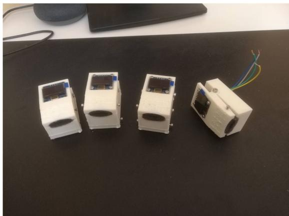
**Fig. 2** The four pulse oximeters at final stages of production
