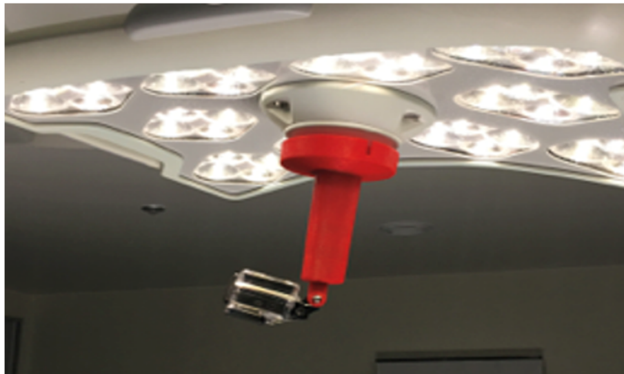
Fig. 3 Reverse engineering. Sterilizable surgical light handle with camera attachment. Date, 2016
