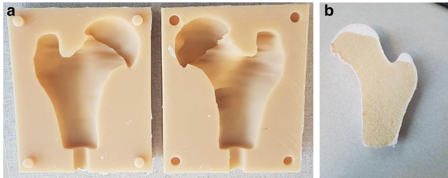
**Fig. 6** Bone models were created using urethane rubber mold and two different urethane casting resins; **a.** The two halves of the urethane rubber mold; **b.** example bone model cut in half to demonstrate the semi-rigid shell and porous foam mimicking real bone structure
