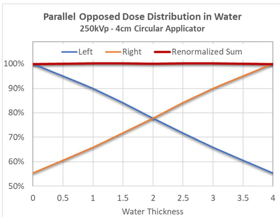
Fig. 3 Parallel opposed Dose Distribution of 250KeV photons in water phantom
