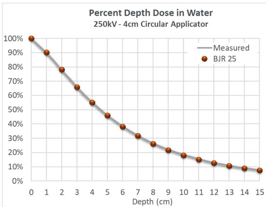
**Fig. 1** Institute verification of percentage depth dose of 250KeV photon beam in water phantom
