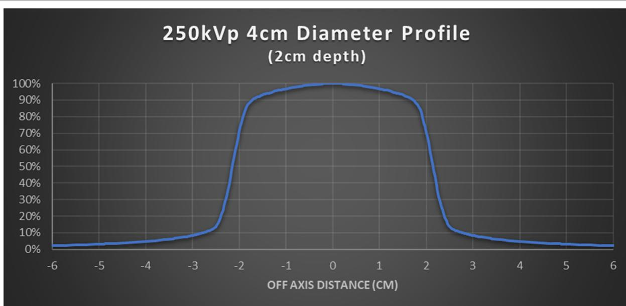
**Fig. 2** Beam profile of 250KeV photon at 2 cm depth of wax
